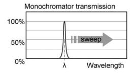
Essentially, the OSA specifications describe the performance of this measuring method. They describe for example; the accuracy, shape, speed and repeatability of the sweeping bandpass filter, but also the accuracy and linearity of the photodetector circuit.
