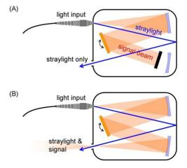
The stray light contribution is measured by blocking the signal beam, see Figure (A). This allows only stray light to exit the monochromator and reach the photodetector.
