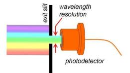
A high resolution (narrow exit slit) in combination with a narrow core input fibre is important to resolve fine spectral detail.
