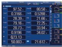
Typical measurement of power value (P1), plus (+) side (P+pk) and minus (-) side (P-pk) of max. power peak value
