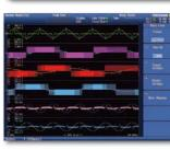
A high resolution display makes is possible to split the waveform display into up to 6 split screens. This makes it possible to split the display of signals between the input and output of a three-phase inverter and display them simultaneously.
