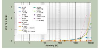
Total power error with rated range input for an arbitrary power factor (at 50/60 Hz)
