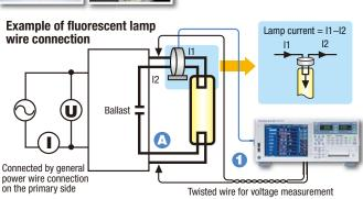
Lamp current can be obtained either by measuring the output of a wide range current sensor as shown in the figure, or by obtaining the differential current using computation (delta computation function).
