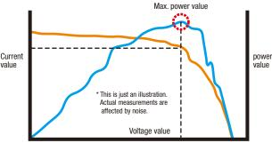
Typical voltage, current, and power measurements in MPPT contro
