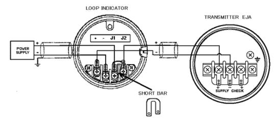
Figure 4.1 General-use Type wiring examples
