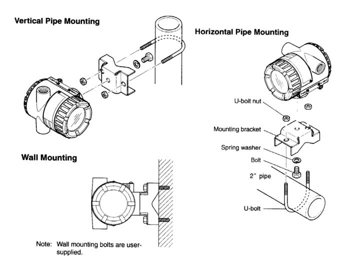
**Figure 3.1 Mounting configurations**
