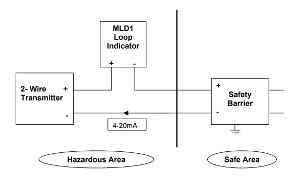
Figure 4.2 Intrinsically Safe Type example
