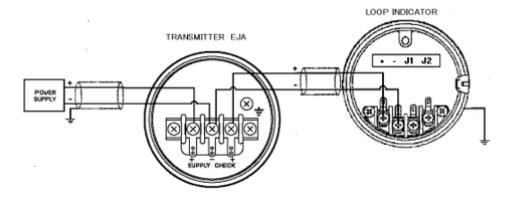
The following is another wiring example of the MLD1 Loop Indicator connected to an EJA Pressure Transmitter (Note: The EJA Transmitter below can be replaced with any 4-20mA 2 wire device.
