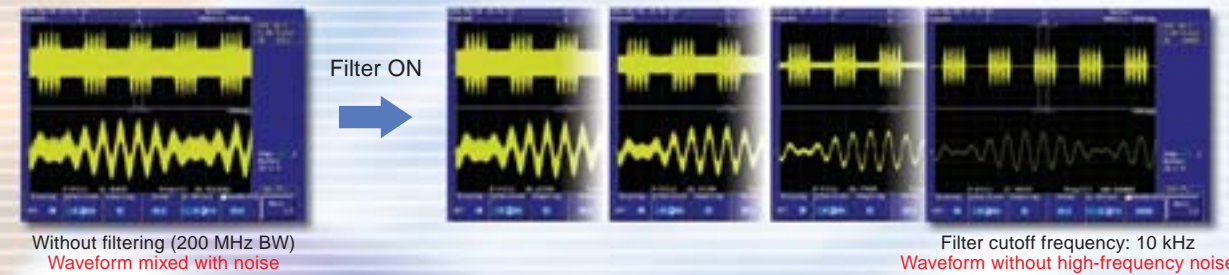
Data Stream Engine II with internal digital filters
