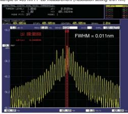
Higher resolution measurement is possible in 400 to 470 nm range.
